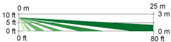
Side View Optional Barrier Coverage: (OMB77) 25 m x 5 m (80 ft x 16 ft)
